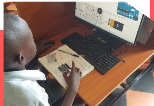
Figure 3: A student physically developing a robot solution after running a successful simulation using Tinkercad
